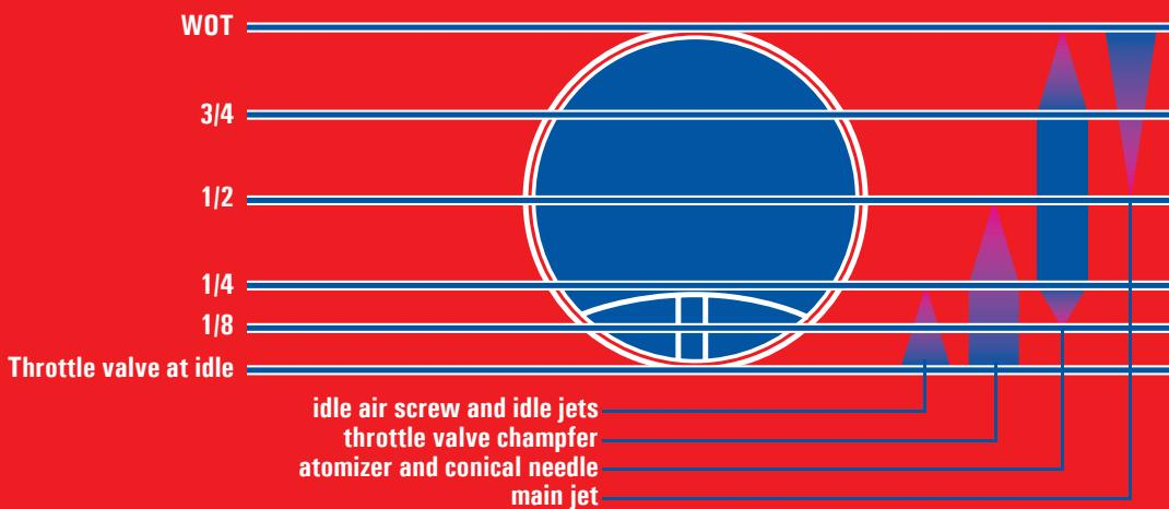
The above picture represents the choke and shows the influence of the different components as far as the throttle gas opening is concerned; it's just indicative and it's however a function of the combination of the different components and of the geometrical features of the conical needle.
